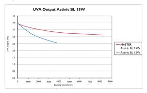
Thanks to the new environmental-friendly water based phosphor technology, the UVA output maintenance and lifetime have been significantly improved. As a result, you can be sure that the lamps will provide maximum and reliable performance during the complete insect season, helping to safeguard a hygienic environment.
