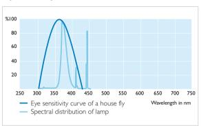
The eyes of insects are sensitive to certain UV wavelengths of the light spectrum. Philips MASTER Actinic BL lamps perfectly match the eye sensitivity of moving houseflies and in this way attract more insects.
