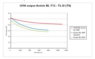
The TL-D (T8) types offer a higher initial UV output of 11% and also better maintenance of this output. This means that the absolute output of a MASTER TL-D lamp after 11,000 burning hours will be the same as a T12 lamp after 1,750 burning hours. Next to this, the UVA brightness of the TL-D version has been improved with 67% compared with the T12 lamp. As a result, you can rely on a maximum performing system during the complete insect season, helping to safeguard a hygienic environment.
