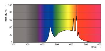
Spectral Power Distribution Colour - MASLEDspot VLE D 6.2-80W GU10 940 36D UK
