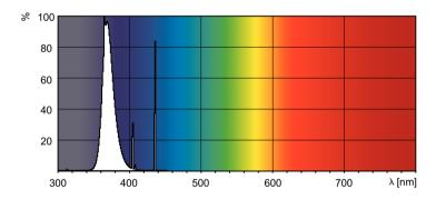
Spectral Power Distribution Colour - Insect PL-L 36W /10
